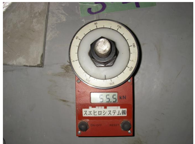
<Anchor pull-out test>
