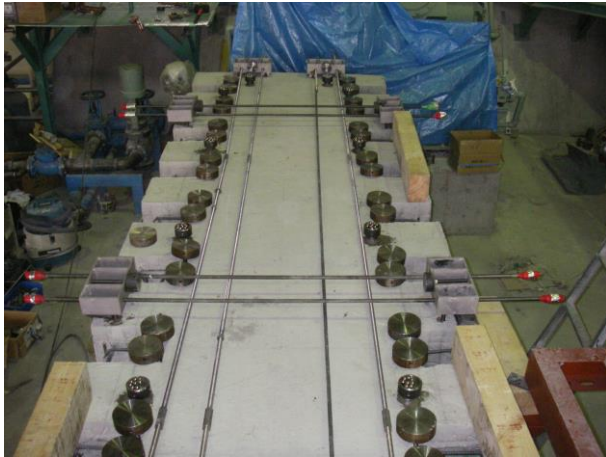
Arrangement of anchor-integrated liners for 9.5-ton engine
