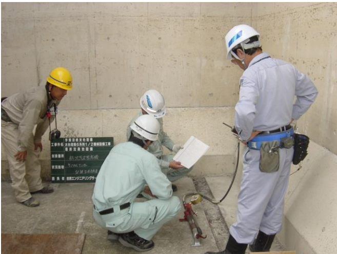
<Test of M16 new-type Deflective Anchor Bolt in the presence of bureau staff>
